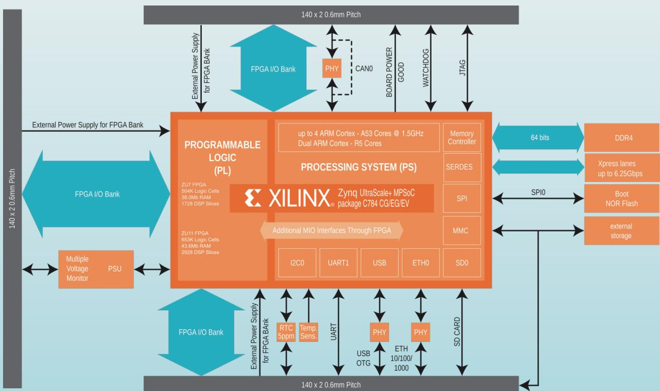
**CPU** up to 4 ARM Cortex-A53 ZYNQ @ up to 1.5GHz
