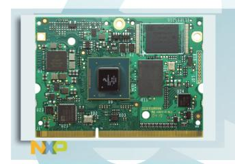
NXP i.MX8M SOM is the new top-class Quad Core ARM Cortex-A53 CPU module by DAVE Embedded Systems, based on the recent NXP i.MX8M application processor. Thanks to this solution, customers have the chance to save time and resources by using a compact solution that permits to reach scalable performances that perfectly fits the application requirements avoiding complexities on the carrier board.
